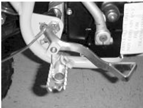
Figure 3, adjust brake lever free height
